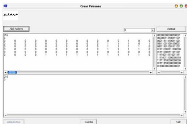
Fig. 3. Building patters from .gif files. In the top left the original word is shown; the map bit at the right shows the normalized pattern of the first character.
