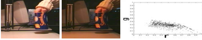
Fig. 1. Example frames of a sequence with time-varying color illuminant and its corresponding color distributions (in normalized rg color space).
