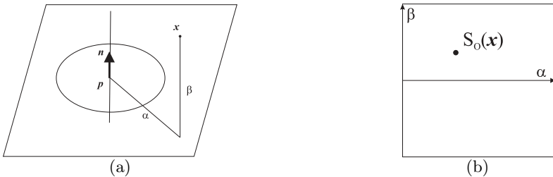
Fig. 1. Given an oriented point \langle \mathbf{p}, \mathbf{n} \rangle on the object surface, a generic point \mathbf{x} is mapped on point [\alpha, \beta] on the spin map, being [\alpha, \beta] the radial distance and the elevation of \mathbf{x} w.r.t. to \langle \mathbf{p}, \mathbf{n} \rangle . a) the object centred 3D coordinates system, and b) the spin map coordinate system.
